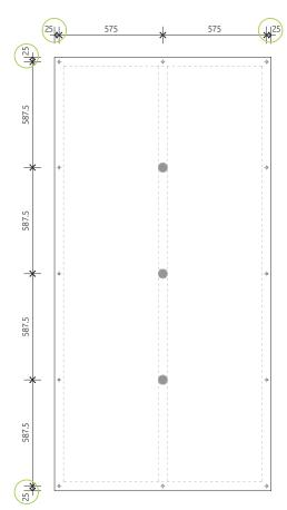
Walls: 25mm 2400 x 1200mm 2390 x 1190mm (adjust fixings in panel corners to 20mm)
