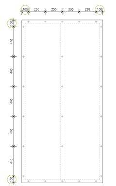
2390 x 1190mm (adjust fixings in panel corners to 95mm and 195mm)
